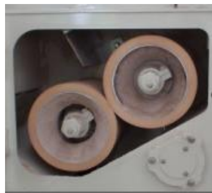
Fig. 16. Rubber roll husker. (Courtesy of Satake Engineering, Ltd.)
