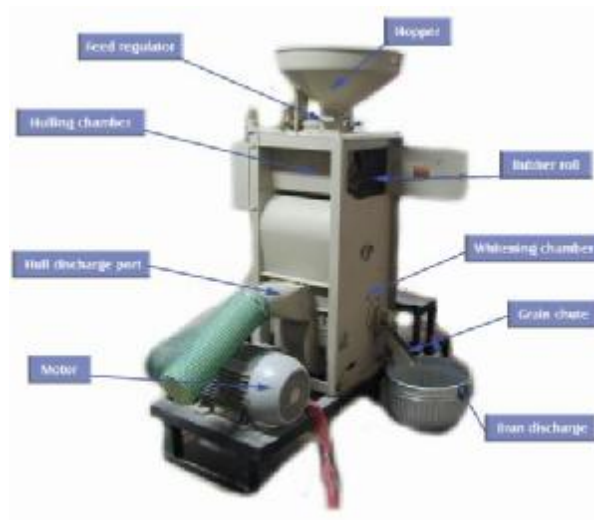
Fig. 3 Modern small-capacity rice mill.
