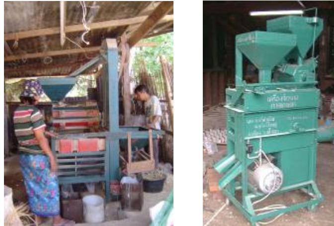
Fig. 5 Village rice mill with single horizontal abrasive roll.
