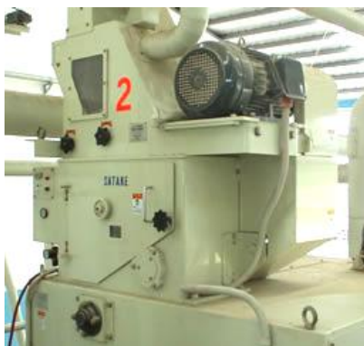
Fig. 16. Rubber roll husker. (Courtesy of Satake Engineering, Ltd.)
