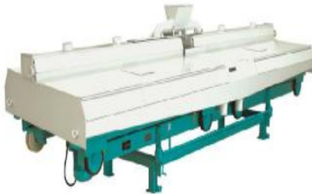
Fig. 21. Compartment-type paddy separator. (BUHLER: DNTB)
